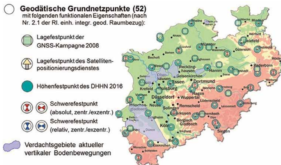
Fig. 4: Geodetic Reference Network Points with their functional characteristics, using North Rhine-Westphalia as an example
