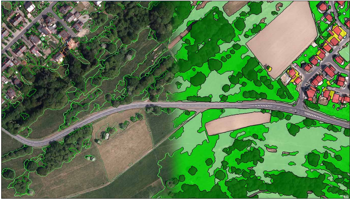
Fig. 15: Image-based classification of landscape elements on the basis of DOP, DOM and DGM data
