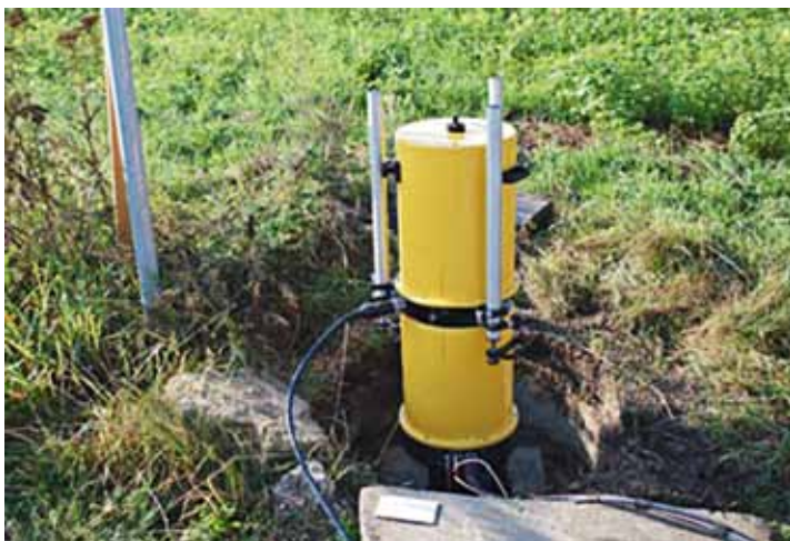
Fig. 4: Absolute gravimeter A-10 on GGP Wallenhorst, Lower Saxony
