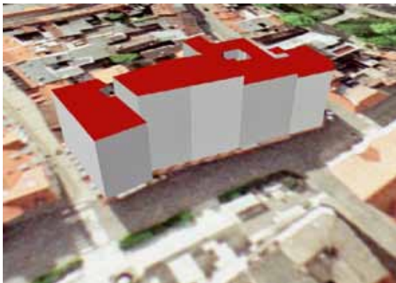
Fig. 9: Level of Detail – LoD 1 (block model from 2013)
