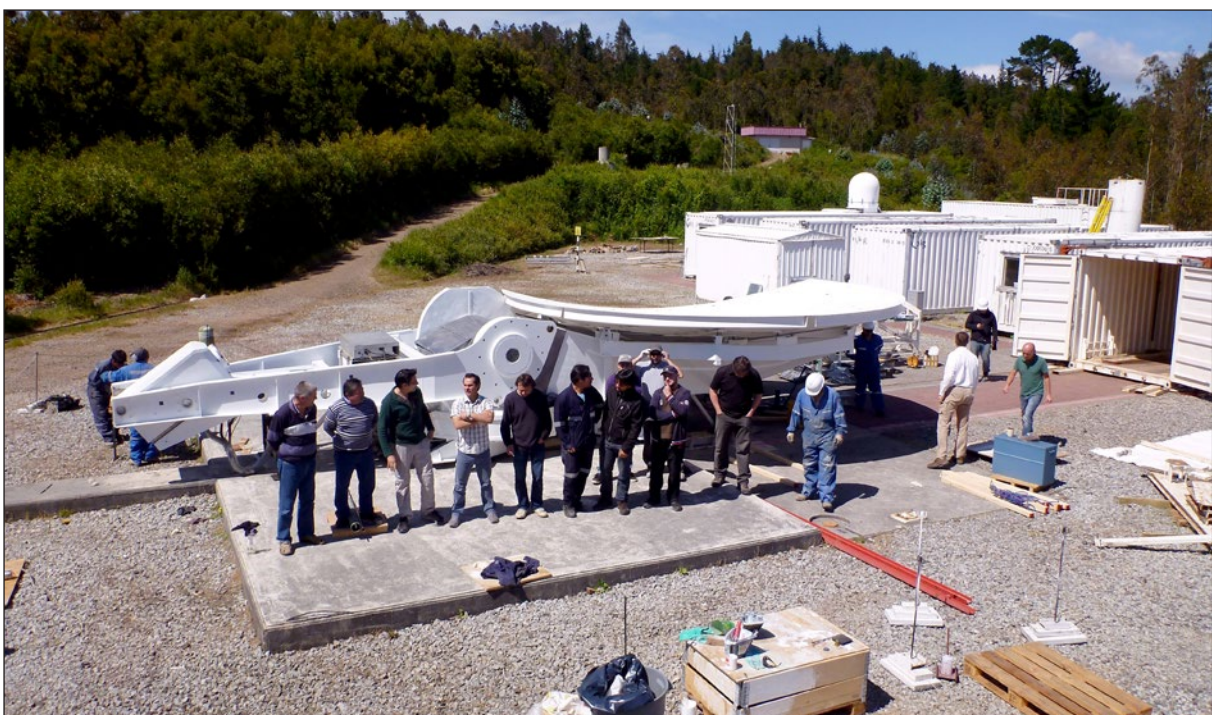
Fig 4: The radio telescope is "folded up" and ready for stowing.
