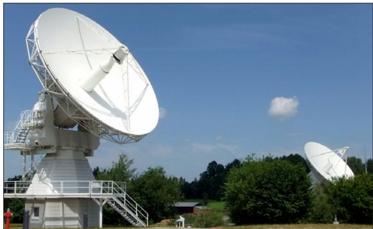
Fig 3: Synchronous operation – the 13.2m TWIN radio telescope TTW1 (foreground, left) and the 20-metre RTW (background) simultaneously measure radio sources (quasars).
