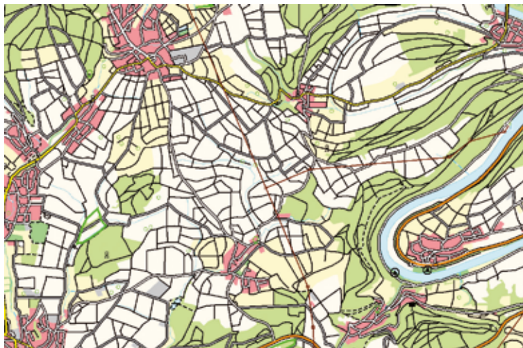
Fig. 6: The DLM50 after automatic cartographic generalisation with presentation objects
