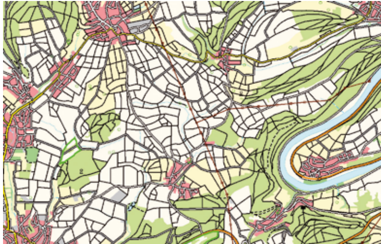
Fig. 5: The DLM50 before automatic cartographic generalisation without presentation objects
