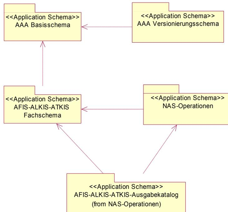
*Figure 44: UML package "NAS-operations" in the context of application schema components*
