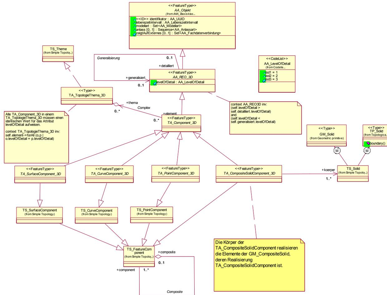
Figure 14: Summary of the 3D basic classes in the standardised Spatial Schema
