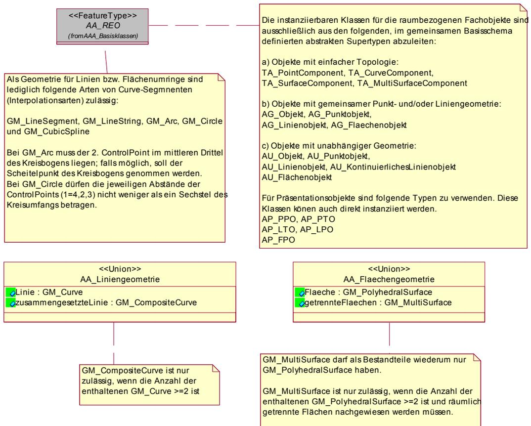
Figure 13: Restrictions concerning geometry and instantiable classes
