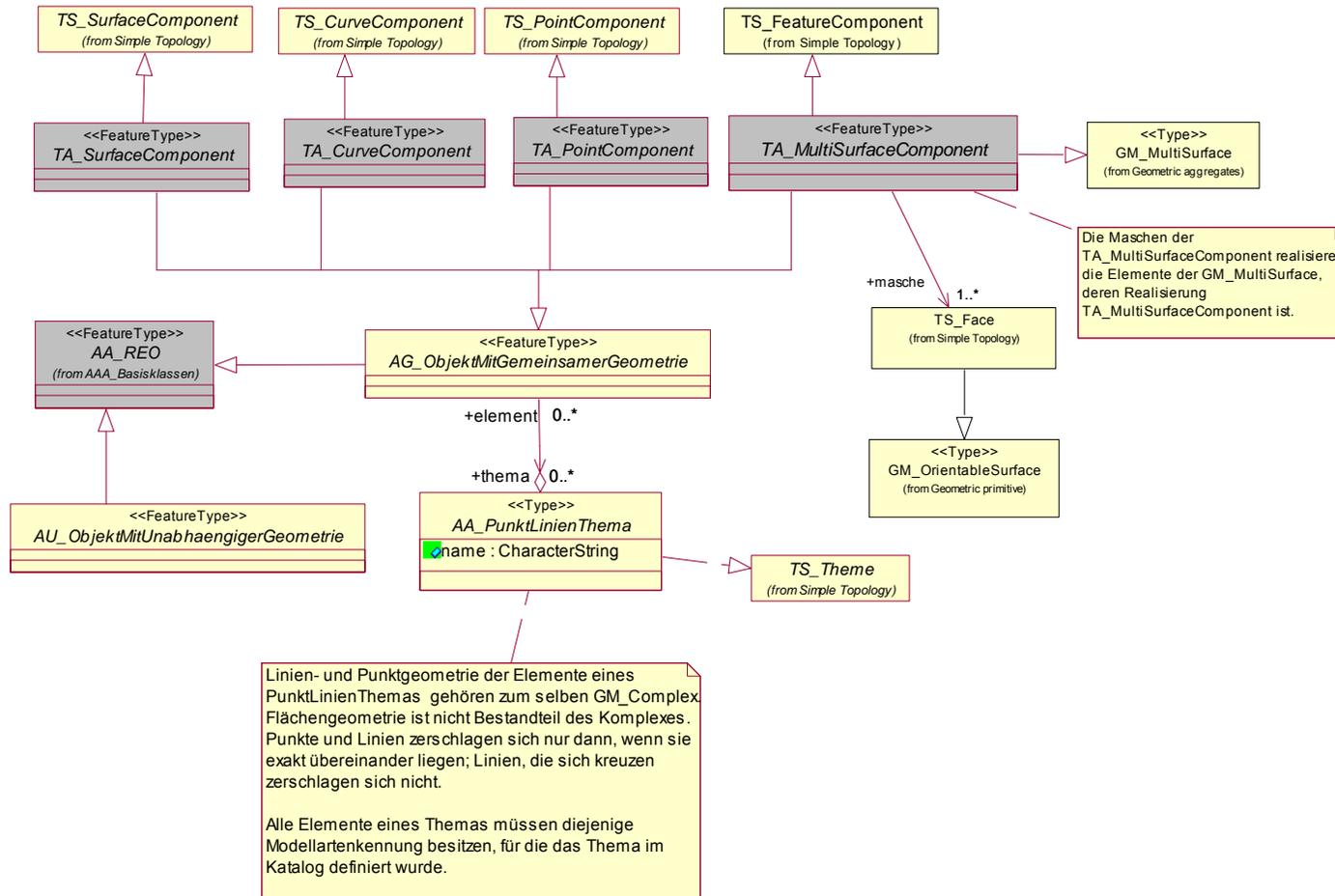
Figure 12: Summary of the enhancements to the standardised Spatial Schema required by AFIS-ALKIS-ATKIS
