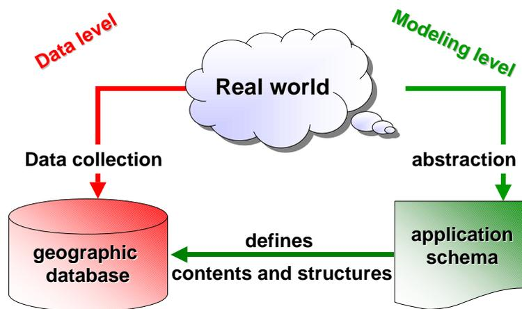
Figure 2: The role of the application schema
