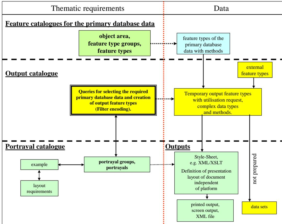
Figure 36: ALKIS output schema
