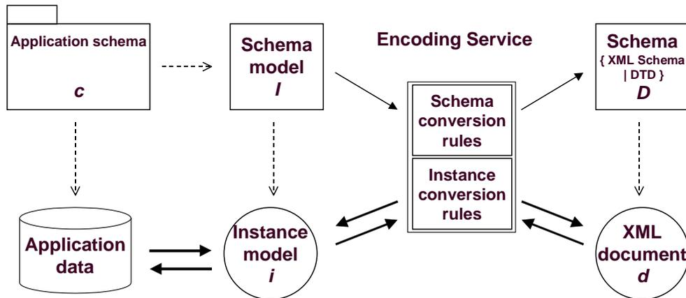
Figure 42: XML based encoding rules in accordance with ISO 19118
