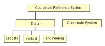
system consists of two components, the "datum" and the "coordinate system" (see sketch).
