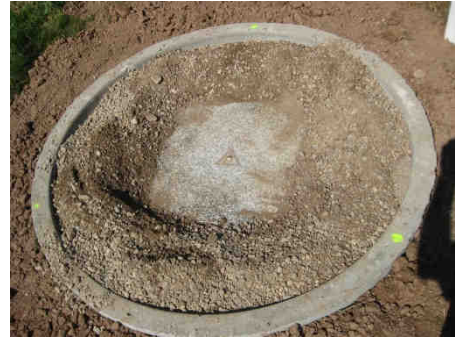
Gravimeterplatte in Betonring
